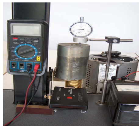
Figure 3. Experimental stand for the study of on-load operation of the paraffin electromechanical actuators
